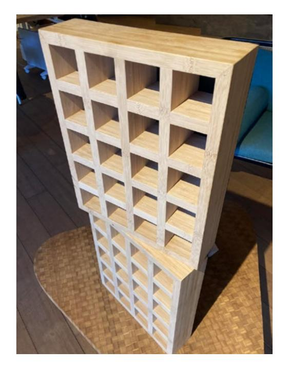
Sample: The first engineered bamboo lattice wall sample prepared for InOne Projects
